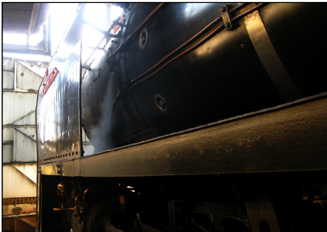
P01 - 15F 3046's new external compressed air connection for the built-in draft ring blower. (Here it was being used for a slow, controlled boiler depressurisation.)
