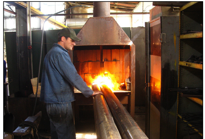
P02 - The 15CA's new boiler flues being heated in the forge for annealing. These would be left alone to air cool. We had four youngsters moving these with woven slings
