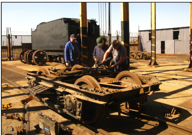
P03 - A donor bar frame-style bogie being serviced and upgraded to be used under Sandstone's Locomotion Coach. (Which will be moving to Bloemfontein soon.)
