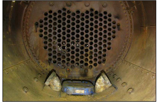
P04 - Class 6A 473 Charlotte's simple front tube plate after having had all the boiler tubes removed.
