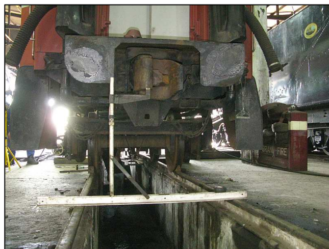
P02 - An original coupler height gauge in use to get the ride heights standardised on the Locomotion Coach.
